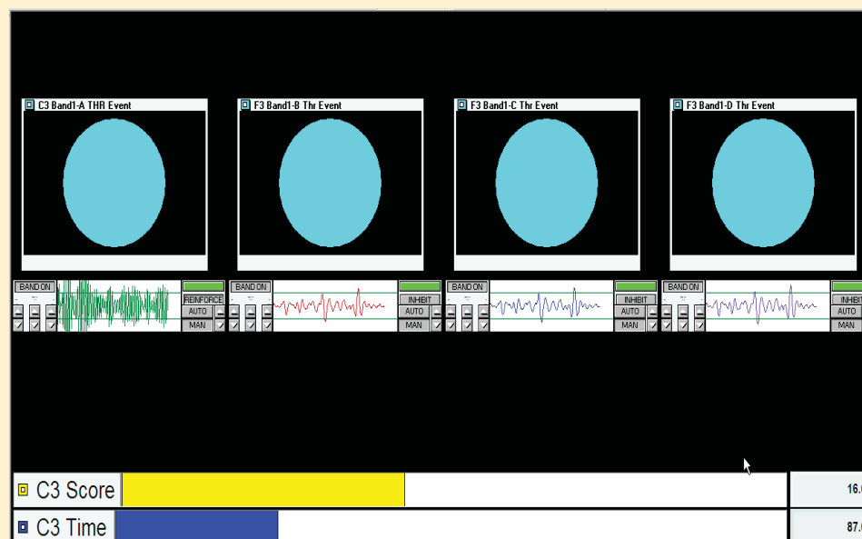
FIGURE 7. Primary display used in our sensorimotor rhythm biofeedback program. The display conforms strictly to operant conditioning principles while still promoting cognitive engagement in the human subject. Reward here is for two different EEG frequencies at two different cortical sites. The far left “green” site shows reinforced 12- to 15-Hz band-pass activity at the C3 electrode site. Low-frequency suppression of abnormal 3- to 5-Hz slow activity at Fz is addressed here through “successive approximation” and consumes the final three display units from left to right. See text for more details. Display results are for the subject depicted in Figure 6.
