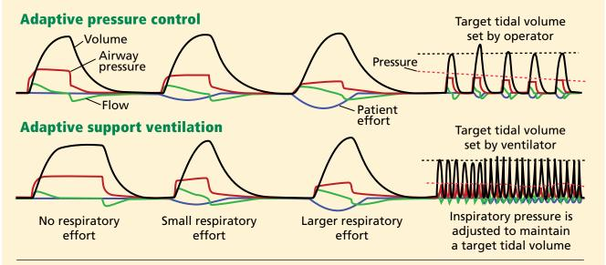
FIGURE 2. A machine in adaptive pressure control mode (top) adjusts the inspiratory pressure to maintain a set tidal volume. Adaptive support ventilation (bottom) automatically selects the appropriate tidal volume and frequency for mandatory breaths and the appropriate tidal volume for spontaneous breaths on the basis of the respiratory system mechanics and the target minute ventilation.
