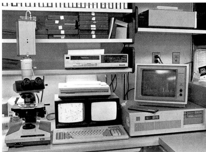
FIGURE 1. Computerized semen analysis instrument.
