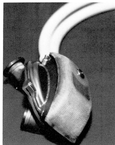
Fig. 9. Integrated CCF/Nimbus left ventricular assist system. The clinical blood pump is machined from titanium.
