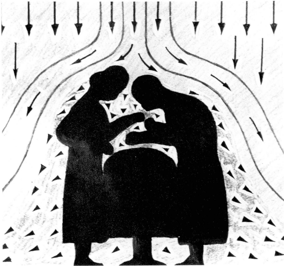
Fig. 6. Practical effect of manual movements near open wound with obstruction to air flow by proximity of bodies of surgical team to the operating table.
