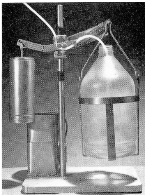
Fig. 3. Collection apparatus with basket, bottle, and counterweight in place.
