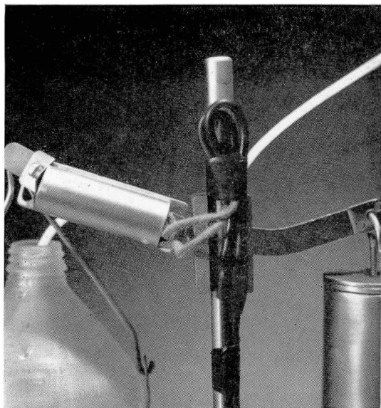
Fig. 5. Mercury-switch circuit control mounted on the balance arm.
