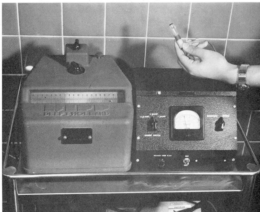
Fig. 2. Photograph of the Clark electrode with its polarograph and galvanometer. The electrode is covered with polyethylene membrane and is fixed in the oxygenator near the outflow end.
